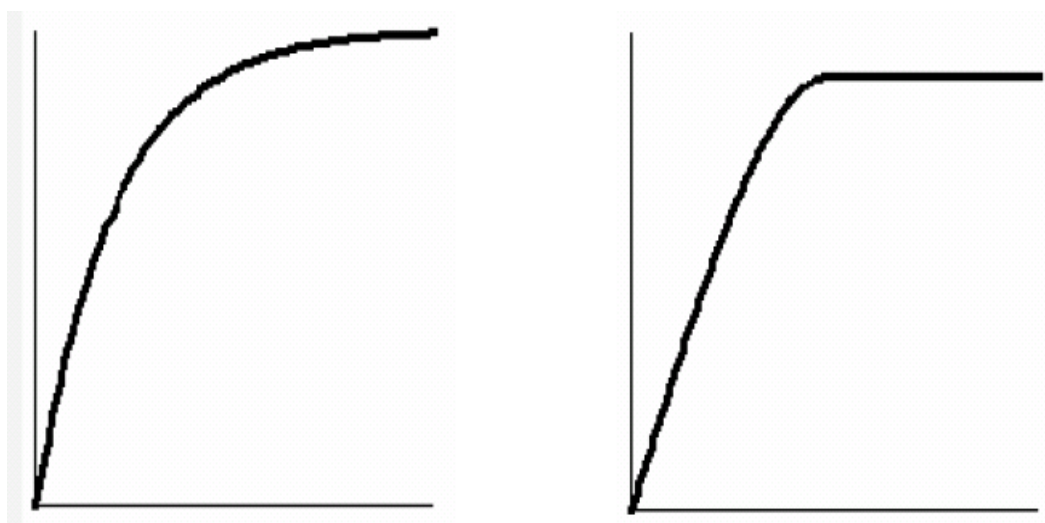
Figure 3.1. Exponential variogram model (left) and spherical variogram model (right)
